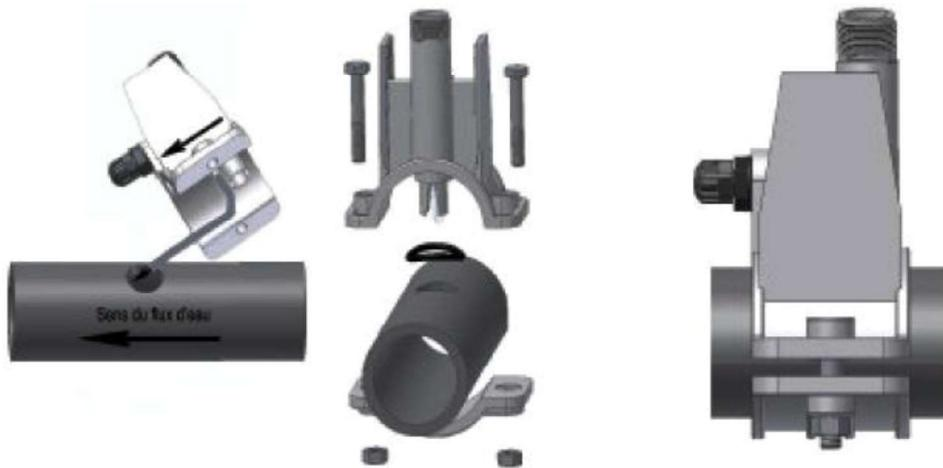
**Fig. 2- Montaje porta sonda**
